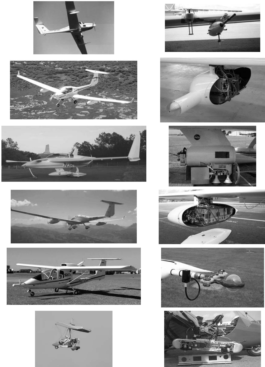
Figure 1 Examples of SERAs (left column) and sensor installations (right column). Top to bottom: Turbulence probe and IR-gas analyser on ARA's G109B (ARA/Flinders University/Adelaide); BAT-probe and INS on ARA's ECO-Dimona; k-Band radar in NOAA's LongEZ (NOAA/Idaho Falls/USA); gas-chromatograph and gas analyser on MetAir's ECO-Dimona (MetAir AG/Switzerland); spectrometers on SDSU's SkyArrow (San Diego State University/USA); aerosol and particle instrumentation on the Research Centre Karlsruhe's Enduro (Research Centre Karlsruhe/Germany).
